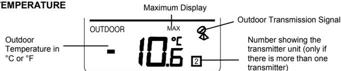
The fifth LCD section shows the outdoor temperature and a transmission signal. A number beside the temperature will also show if more than one transmitter is used.
