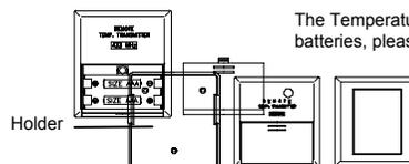
The Temperature Transmitter uses 2 x AAA, IEC, LR3, 1.5V batteries. To install and replace the batteries, please follow the steps below:
