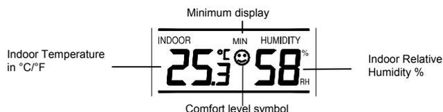
The indoor temperature and humidity are received automatically and displayed on the fourth section of the LCD.
