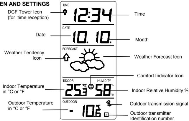
For better distinctness, the LCD screen is split into 5 sections displaying the information for time, date, weather forecast, indoors and outdoors.
