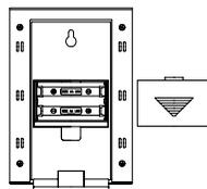
The Weather Station uses 2 x AA, IEC LR6, 1.5V batteries. If the batteries need to be replaced, the battery symbol will appear on the LCD.
