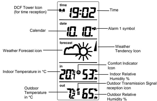
For better distinctness the LCD screen is split into 5 sections displaying the informations for time, date, weather forecast, indoors and outdoors.
