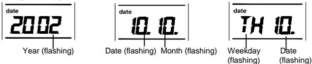
The date default of the Weather station is 1. 1 or TH 1. in the year 1998. Once the radio-controlled time signals are received, the date is automatically updated. However, if the signals are not received, you can adjust the date manually. To do this:
