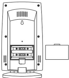
The Weather station uses 2 x AA, IEC LR6, 1.5V batteries. When batteries need to be replaced, the battery symbol will appear on the LCD. To install and replace the batteries, please follow the steps below:
