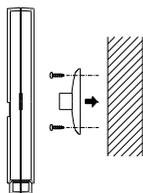
The Transmitter is supplied with a holder that may be attached to a wall with the two screws supplied. The Transmitter can also be position on a flat surface by securing the stand to the bottom to the Transmitter. Before securing the transmitter, ensure that the 433MHz signal (outdoor readings) is properly received.
