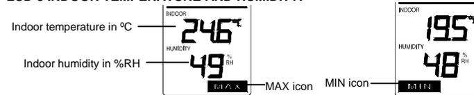
The indoor temperature and humidity are measured and displayed on the third section of the LCD.
