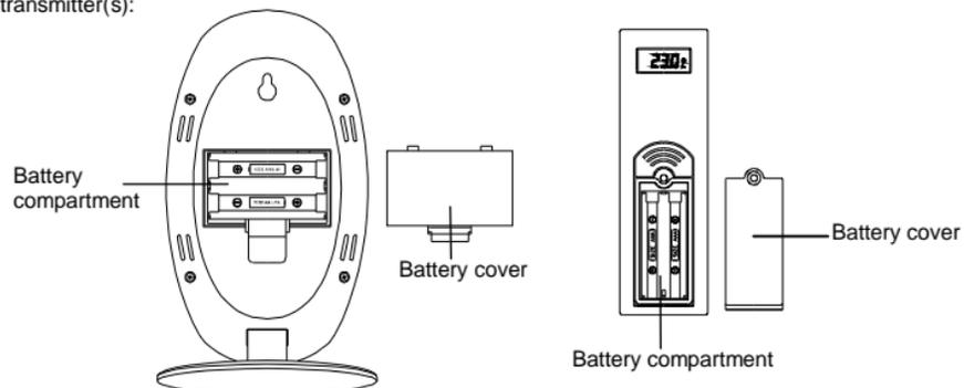
1. First, insert 2 x AA, IEC LR6, 1.5V batteries into the Weather Station. Once the batteries are in place, all segments of the LCD will light up briefly. Then the indoor temperature, the time as --:-- , and the weather icons sun and clouds will be displayed. If the indoor temperature is not displayed after a few
