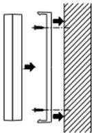
The Outdoor Temperature transmitter is supplied with a holder and three screws for wall mounting. Before securing the transmitter, ensure that the 433MHz signal (outdoor temperature) is properly received.
