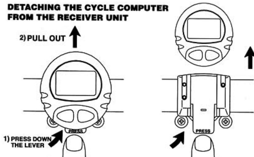
The user is advised to remove the main bikemeter from the Receiver Mounting when not in use to avoid theft and damage during transportation.
